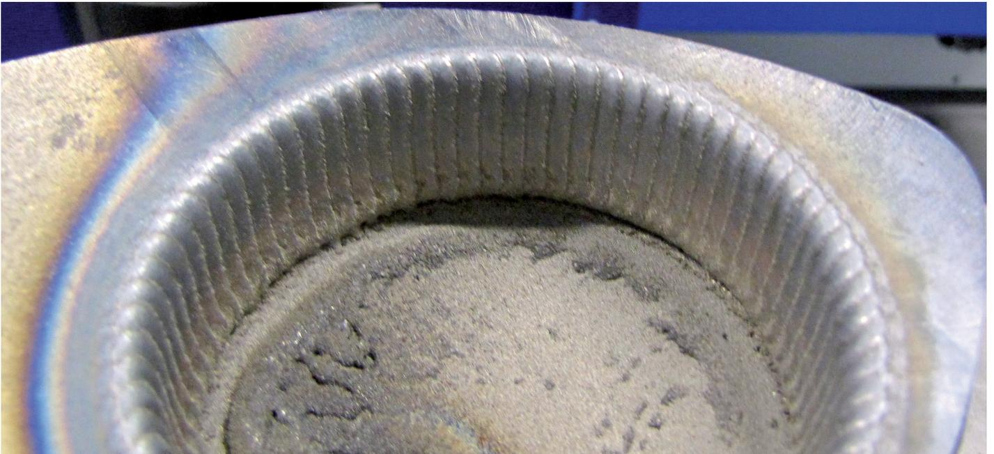
Surface cladding can be carried out on outer and inner diameters.
