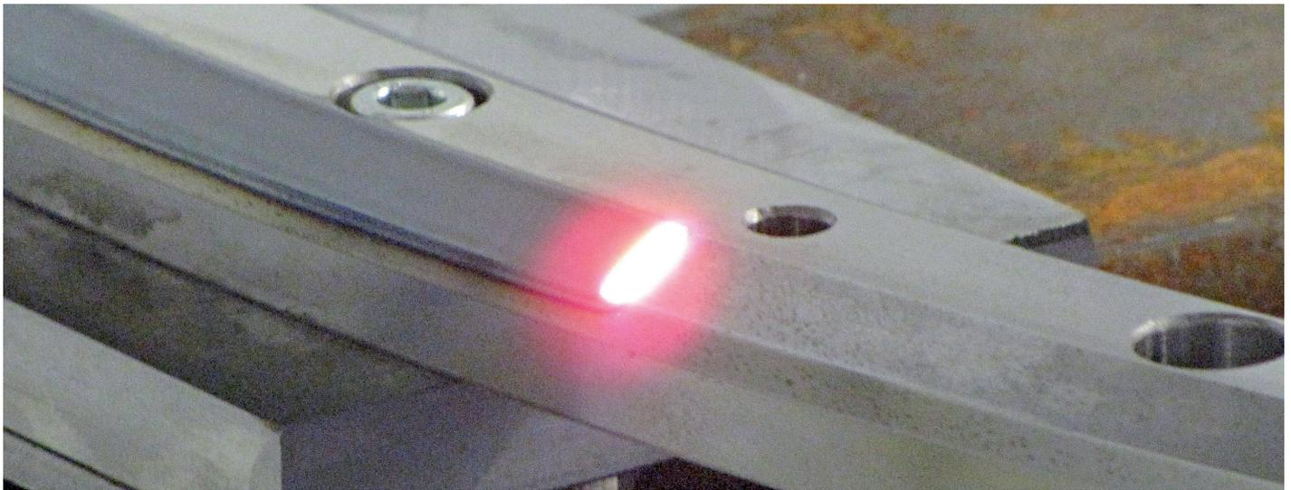
We can make laser hardening on supporting elements of machine tools.
