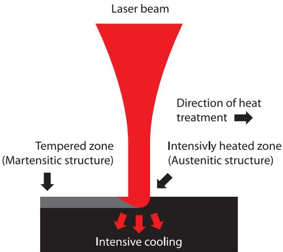
Laser tempering uses the self-cooling effect of the material to create the tempered layers.
