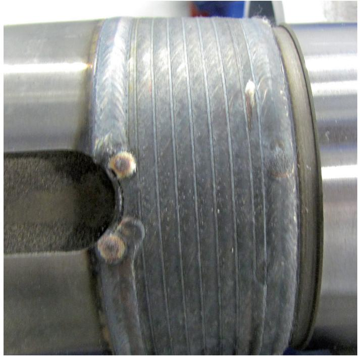
The technology of alloy cladding is suitable for repair of surfaces as well as enhancing of properties of surface layers in terms of increased lubricity, hardness, abrasion-resistance, improved cavitation, corrosion resistance, resistance at high temperatures and pressures, etc.
