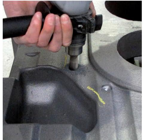
Preparing for weld by drilling
