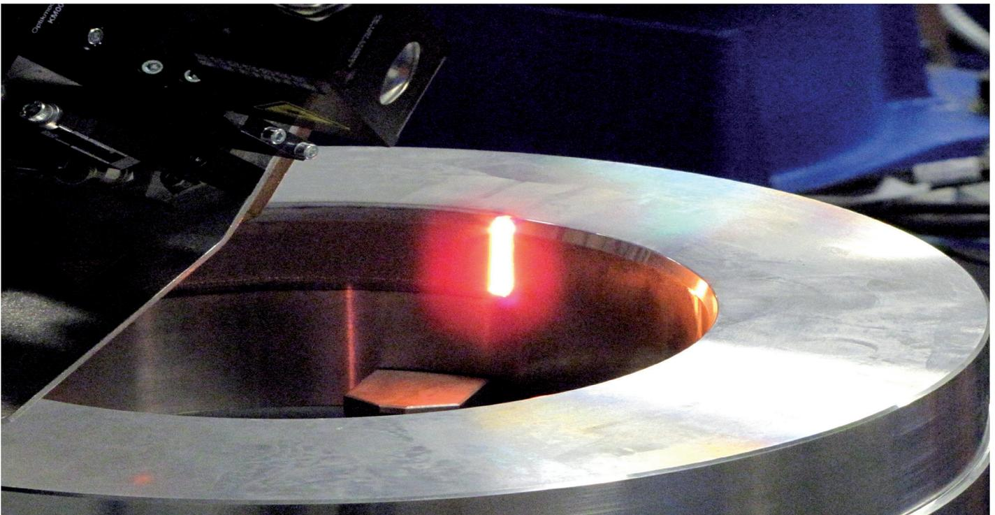
With scanning and focusing of the beam at a distance of 170 mm from the front of the head, we are able to harden cavities with the depth distance of up to 140 mm.
